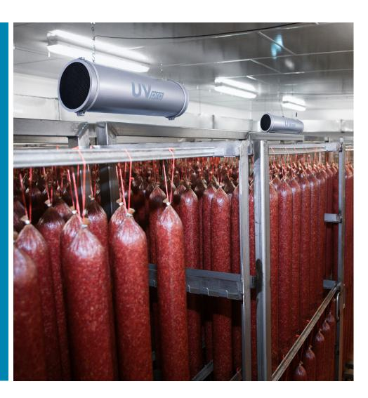
The elimination of resistant germs and mold spores is important, particularly in industrial food production. The UVpro circulating-air purifiers from orca GmbH reliably perform this task. For the manufacture of these purifiers, the company relies on tubes made by JACOB, which are used to house the devices.
